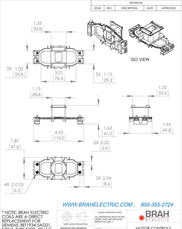
SIRIUS, TYPE B3RT, 42VAC AC 50/60HZ, SUITABLE FOR USE WITH 3RT1033, 3RT1034 CONTACTORS
