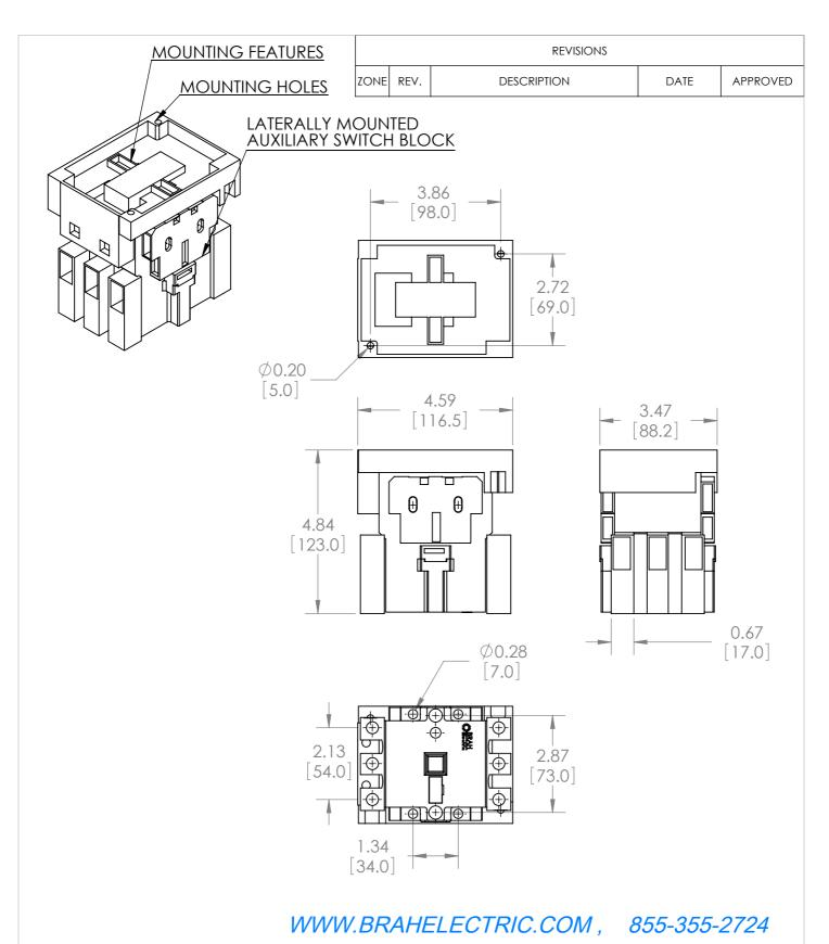
\*NOTE: BRAH ELECTRIC CONTACTOR B3TF4622-0AK6 IS AN AFTERMARKET DIRECT REPLACMENT FOR 3TF4622-0AK6,3TF SERIES. SUITABLE FOR USE WITH 3TF SERIES MOTOR CONTROL **SYSTEMS**
