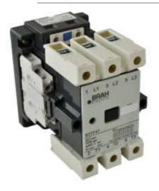
MAGNETIC CONTACTOR PART NO. B3TF4622-0AK6 PART NUMBER – B3TF4622-0AK6: BRAH Electric, aftermarket direct replacement contactors for Siemens 3TF4622-0AK6, World Series, type 3TF, 3P, 3PH, 45A, 600V, 20HP @ 230V, 40HP @ 460V, 50HP @ 575V, complete with 110/120V AC coil, 2 N/O - 2 N/C auxiliary contact, AC magnetic contactor, suitable for use with 3TF series motor control systems
