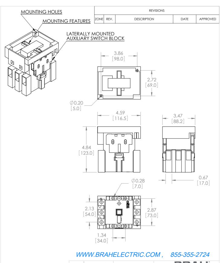
\*NOTE: BRAH ELECTRIC CONTACTOR B3TF4722-0AP6 IS AN AFTERMARKET DIRECT **REPLACMENT FOR 3TF4722-**OAP6,3TF SERIES. SUITABLE FOR USE WITH 3TF SERIES MOTOR CONTROL SYSTEMS
