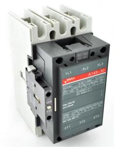
aftermarket direct replacement contactors for ABB A145-30-11-83, A-Line series, type A, 3P, 3PH, 130A, 600V, 50HP @ 240V, 100HP @ 480V, 125HP @ 600V, complete with 48V AC coil, and 1 NO/NC auxiliary contact, AC magnetic contactor, suitable for use with A-Line series motor control systems
