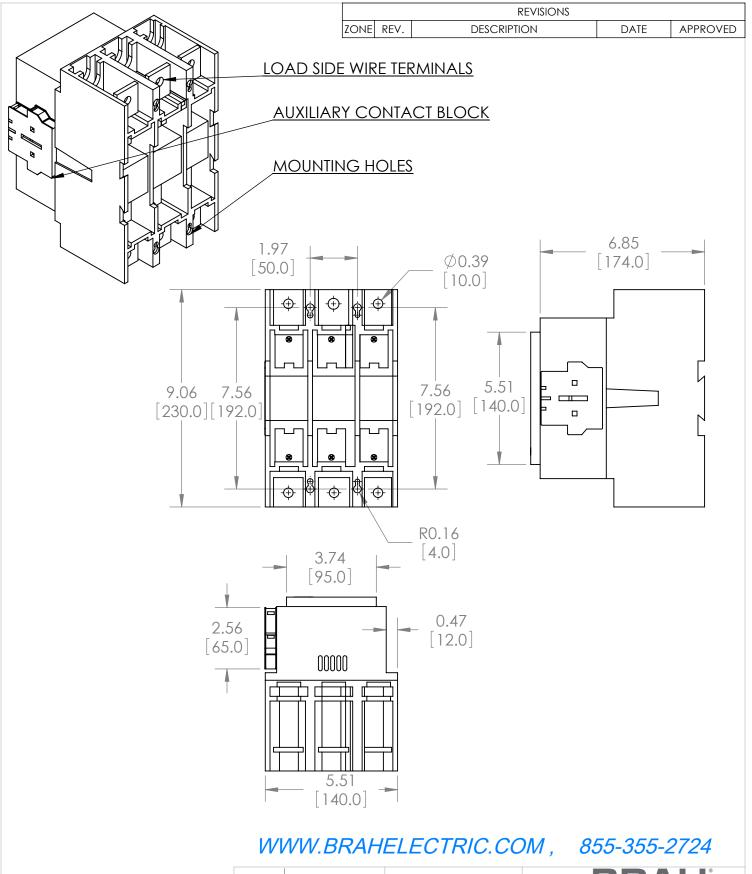
\*NOTE: BRAH ELECTRIC CONTACTOR BA210-30-11-51 IS AN AFTERMARKET DIRECT REPLACMENT FOR A210-30-11-51, A-LINE SERIES. SUITABLE FOR USE WITH A-LINE SERIES MOTOR CONTROL **SYSTEMS**
