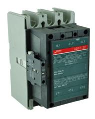
PART NUMBER – BA210-30-11-51: BRAH Electric, aftermarket direct replacement contactors for ABB A210-30-11-51, A-Line series, type A, 3P, 3PH, 192A, 600V, 75HP @ 240V, 150HP @ 480V, 200HP @ 600V, complete with 480V AC coil, and 1 N/O - 1 N/C auxiliary contact, AC magnetic contactor, suitable for use with A-Line series motor control systems
