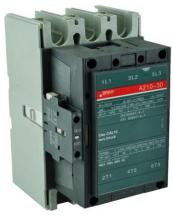
PART NUMBER – BA210-30-11-84: BRAH Electric, aftermarket direct replacement contactors for ABB A210-30-11-84, A-Line series, type A, 3P, 3PH, 192A, 600V, 75HP @ 240V, 150HP @ 480V, 200HP @ 600V, complete with 120V AC coil, and 1 N/O - 1 N/C auxiliary contact, AC magnetic contactor, suitable for use with A-Line series motor control systems
