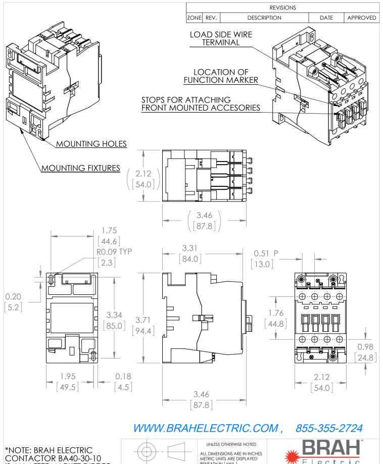
IS AN AFTERMARKET DIRECT REPLACMENT FOR ABB A40-30-10, A-LINE SERIES. SUITABLE FOR USE WITH A-LINE SERIES MOTOR CONTROL SYSTEMS
