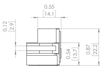
NOTE: BRAH ELECTRIC **COILS ARE A DIRECT** REPLACEMENT FOR GENERAL ELECTRIC, POWER BREAK 1, TYPE TR32,1200 Amp PLUG FOR 3200 Amp CT SENSOR RATING, SUITABLE FOR USE WITH **AKR75 EQUIPPED WITH** MICROVERSA TRIP RMS-9 SOLID STATE ELECTRONIC TRIP UNITS.
